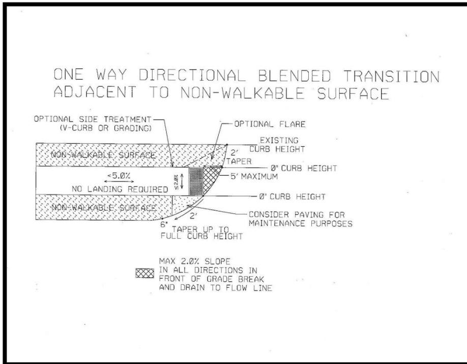
Figure 6: One Way Directional Ramp Adjacent to Non-Walkable Surface
