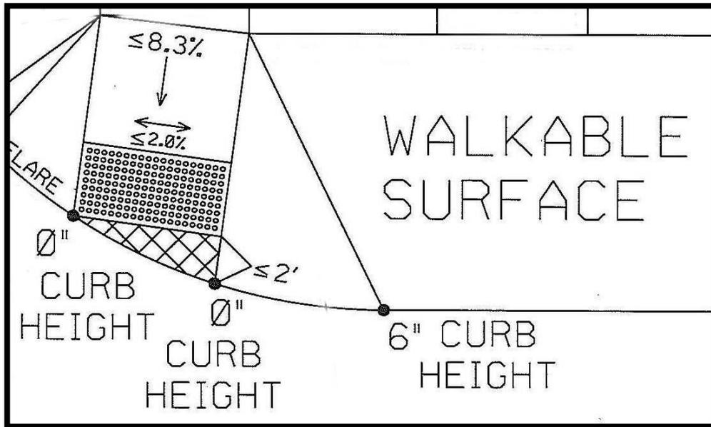
Figure 12: Curb and Gutter – Standard and Pedestrian Access Route
