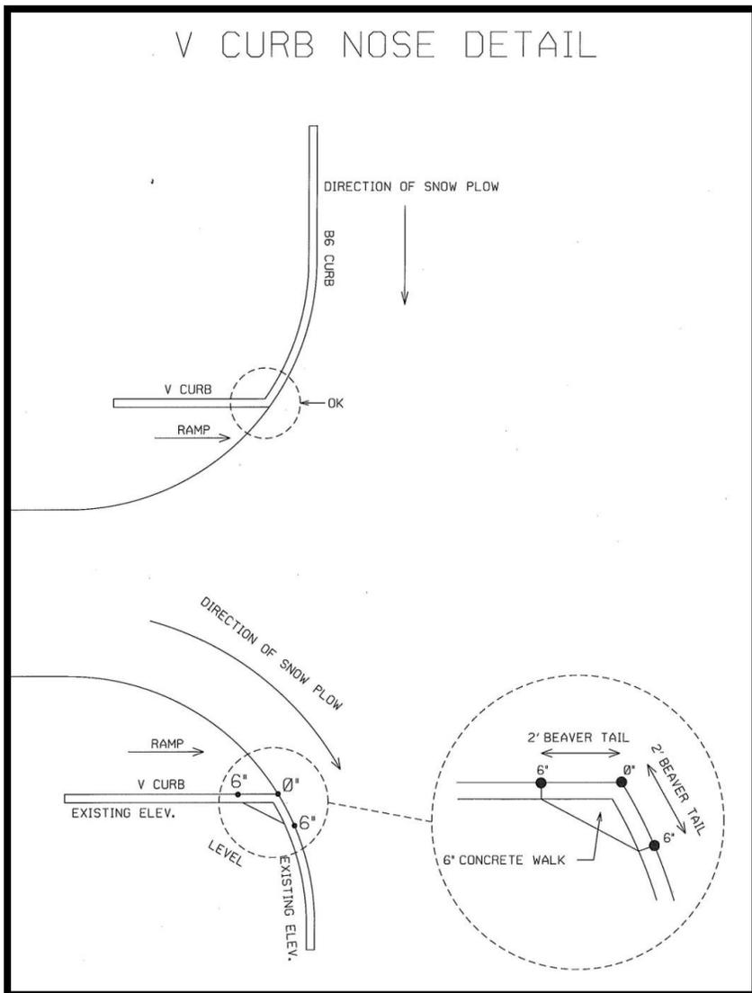
Figure 13: "V" Curb Nose Detail
