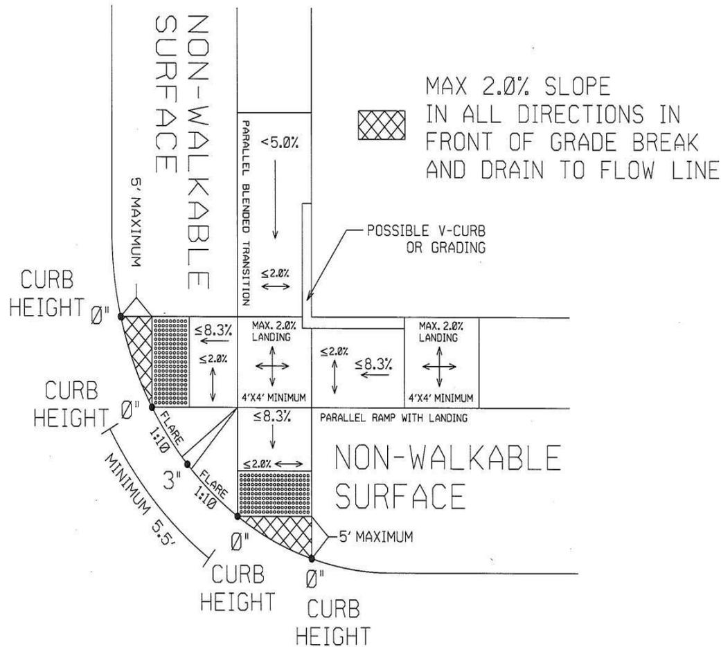
Figure 5: One Way Directional Ramp Adjacent to Curb and Gutter
