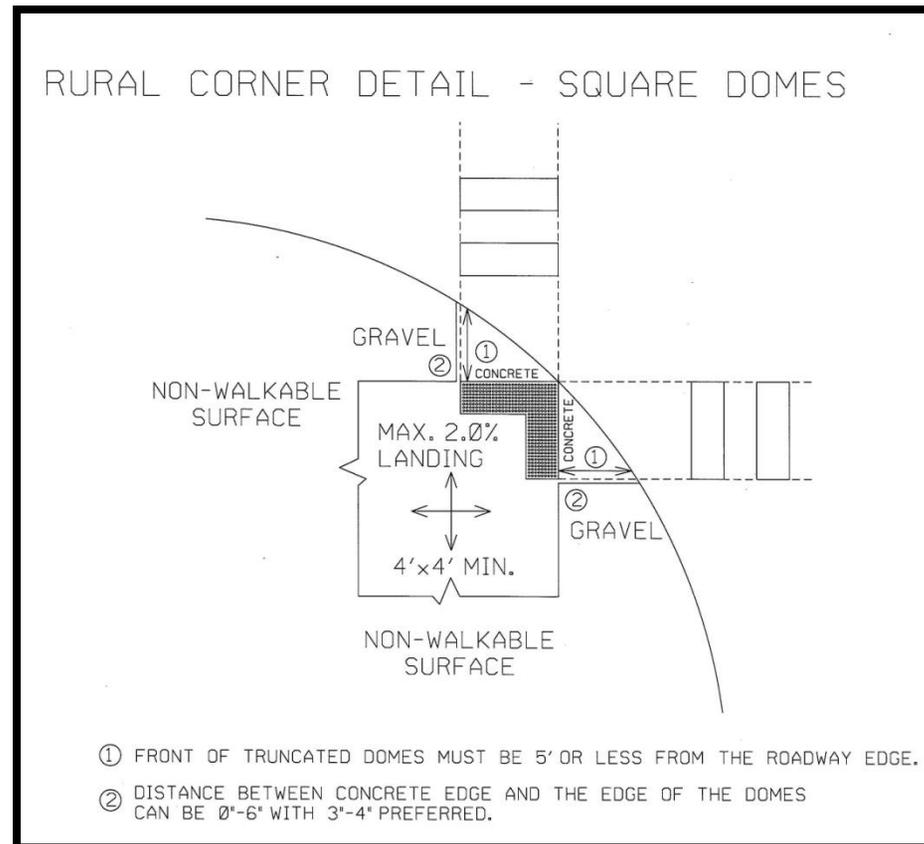
**Figure 15: Flat Landing with Directional Domes**
