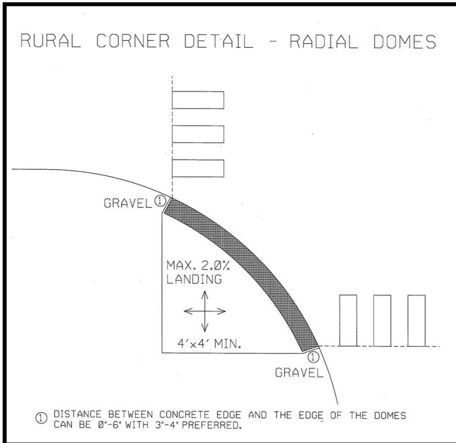
**Figure 16: Flat Landing with Radial Domes**
