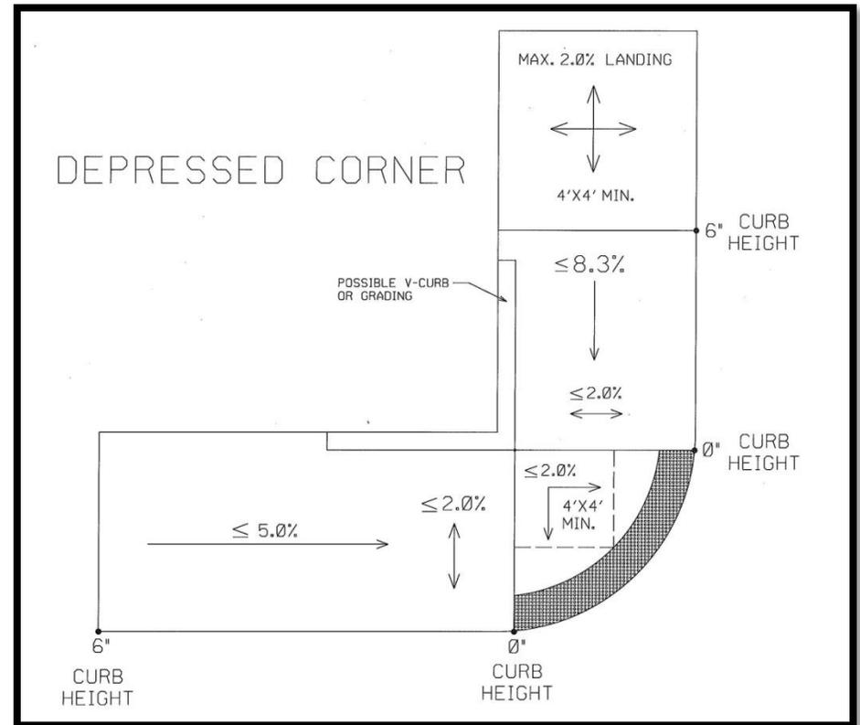
**Figure 8: Depressed Corner Detail**
