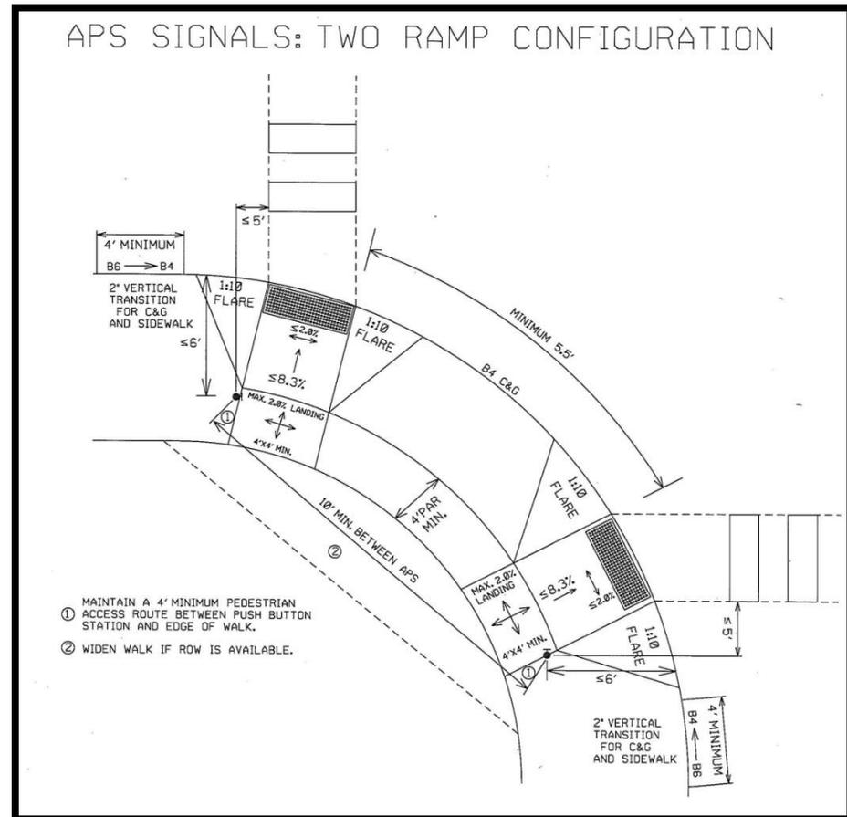
Figure 14: Accessible Pedestrian Signal
