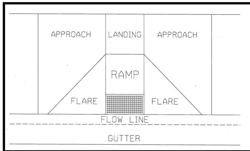
*Figure 1: Curb Ramp Components*
