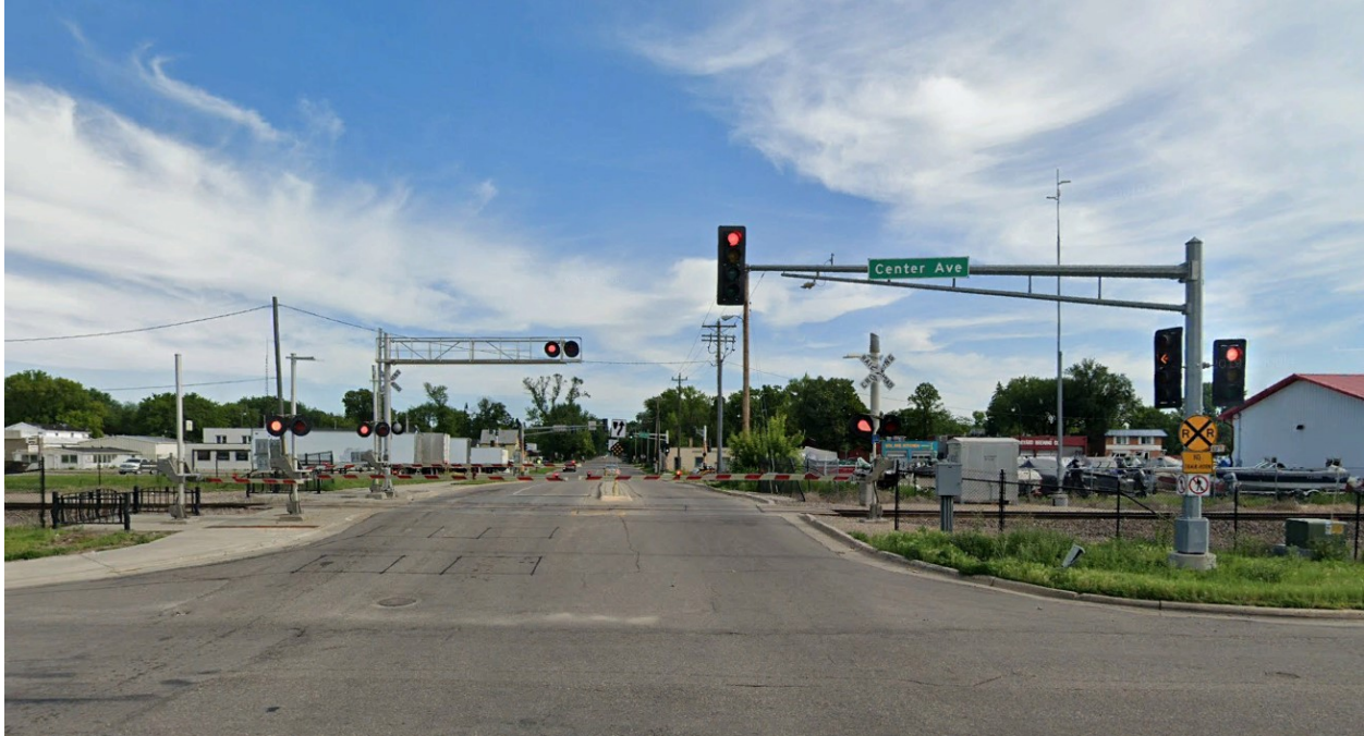
Figure 7. Grade Crossing with Traffic Signal Preemption (Source: AECOM)
