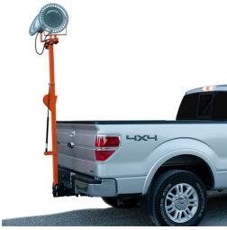
Whether it is in an emergency situation or night-time maintenance operations, it is difficult for the motoring public to see workers on the road. The OptoEngineering Truck Mounted LED Light Tower (TMLT) provides a lighting component that illuminates the work area so that flaggers or workers can be seen by the public.
