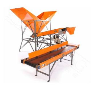
The Burcham High Production Bagger is the only sandbag filling machine on the market today that both fills the sandbag, and sews it shut. The project was submitted by Danny Hoeper and Mark Pederson from District 2. Operating the Burcham Bagger is as simple as lifting a bag to the spout.
