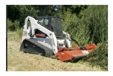
The Bobcat Flail Cutter attachment project was submitted by Jon Beeman and Rick Nacsak in District 6E. The attachment clears brush and small trees while distributing cut materials evenly. It has a cutting width of 79 inches and delivers excellent cutting and mulching action for materials up to three inches in diameter. Specific mowing areas can be done more efficiently.
