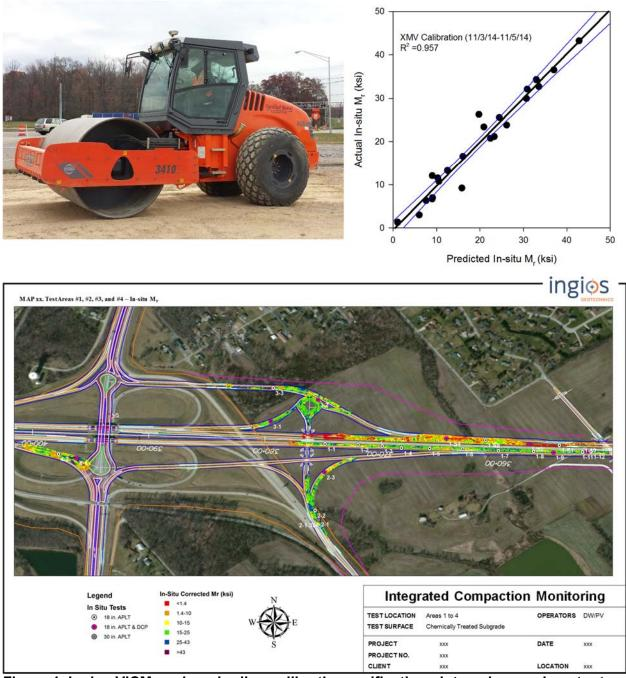
Figure 1. Ingios VICM equipped roller, calibration verification plot, and example output.
