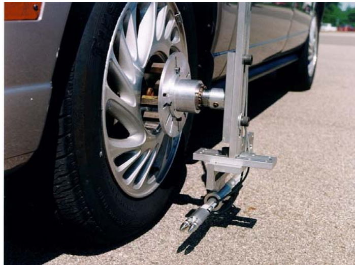
Figure 8. Mounting Arrangement for Sound-Intensity Microphones (12)
