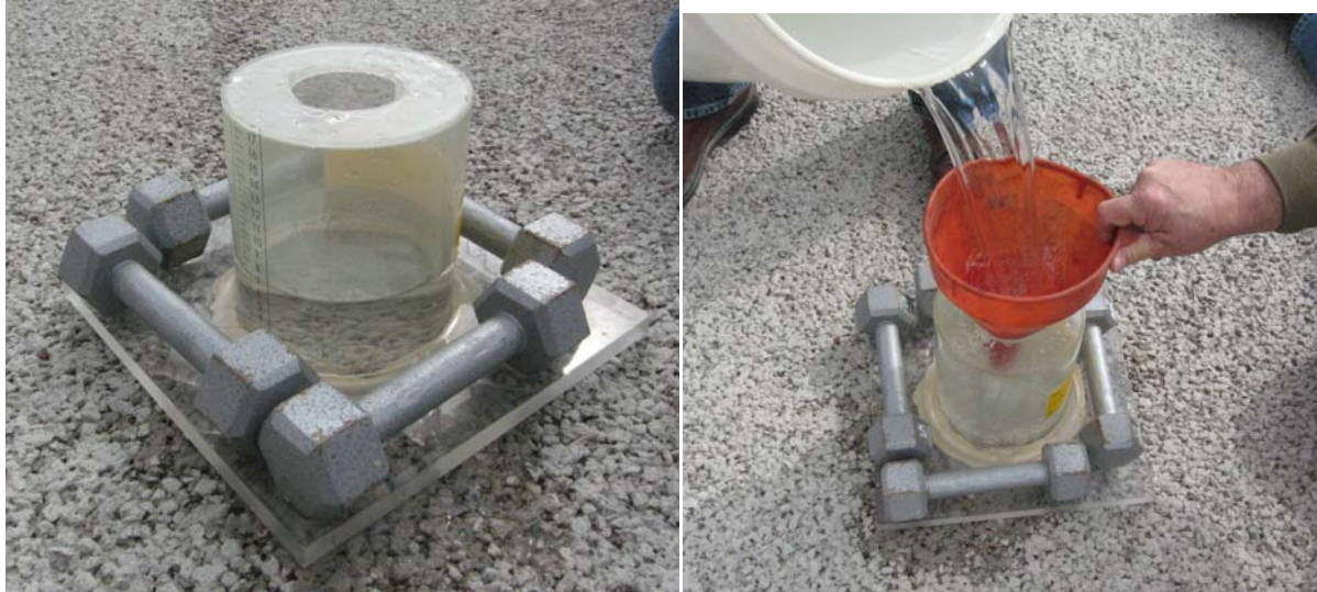
Figure 74. NCAT infiltration test device (2009)
