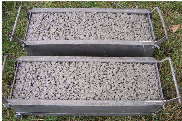
Figure 36. Fresh concrete with no curing compound
