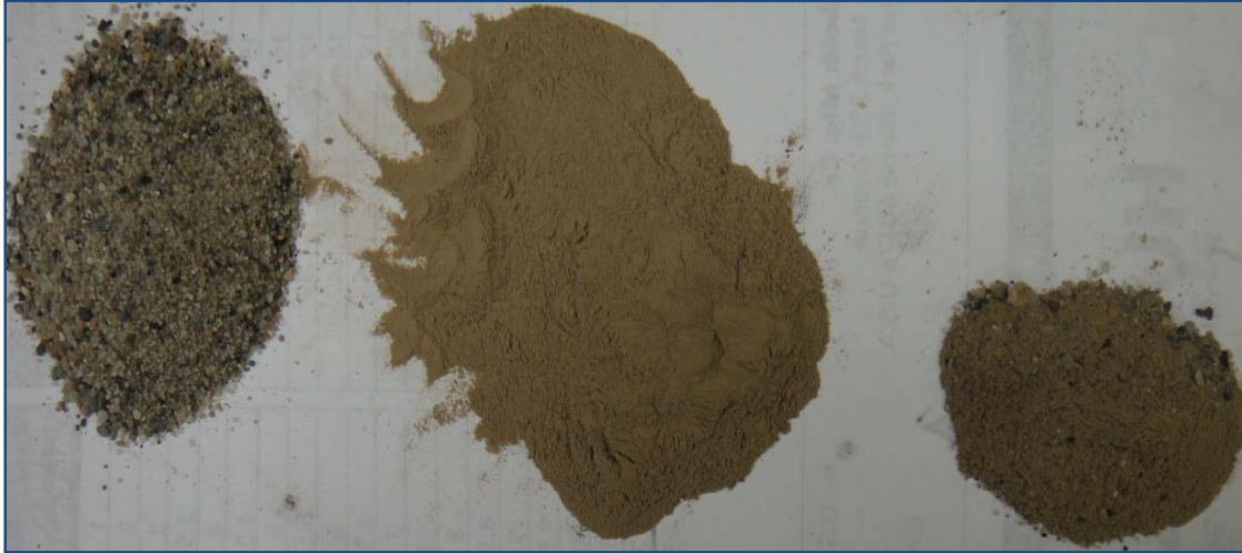
Figure 48. Three sediment materials used: sand (left), silty clay (middle), and silty clay sand (right)
