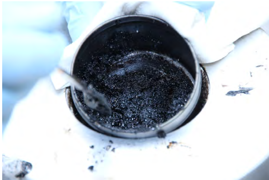
Figure 3.4. Manually mixing glass beads with the asphalt binder to prepare a homogenous mix
