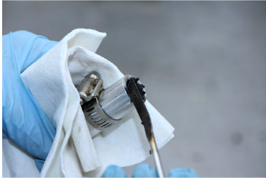
Figure 3.5. Mold being filled with the loose binder-glass bead mix
