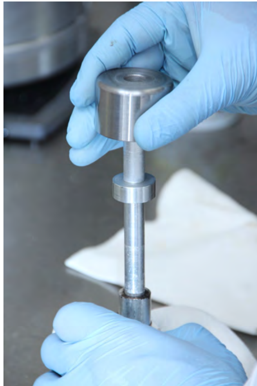
Figure 3.6. Loose mix being compacted using 25 drops of a weight from a specific height
