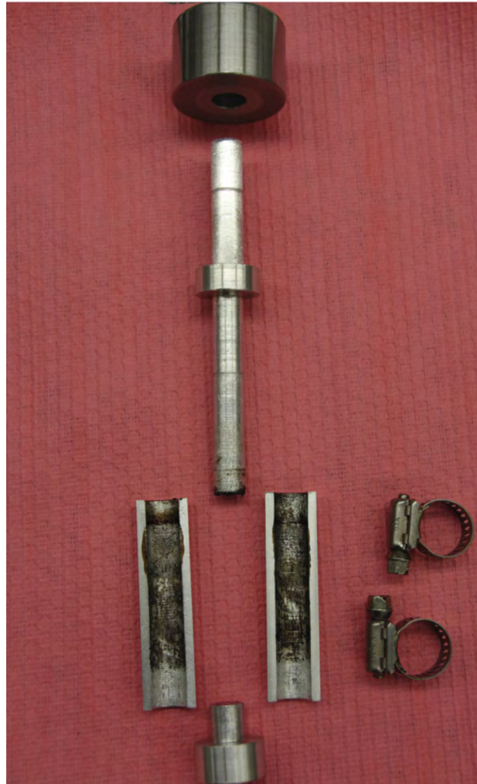
Figure 3.2. Assembly of the compaction mold
