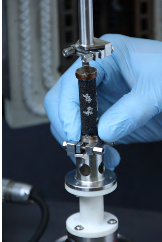
Figure 3.8. Test specimen being mounted on the DSR for testing
