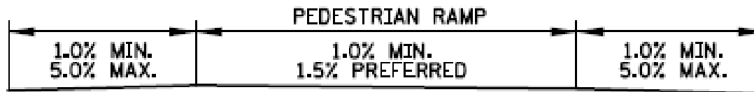
FLOW LINE PROFILE RAISE - FAN
