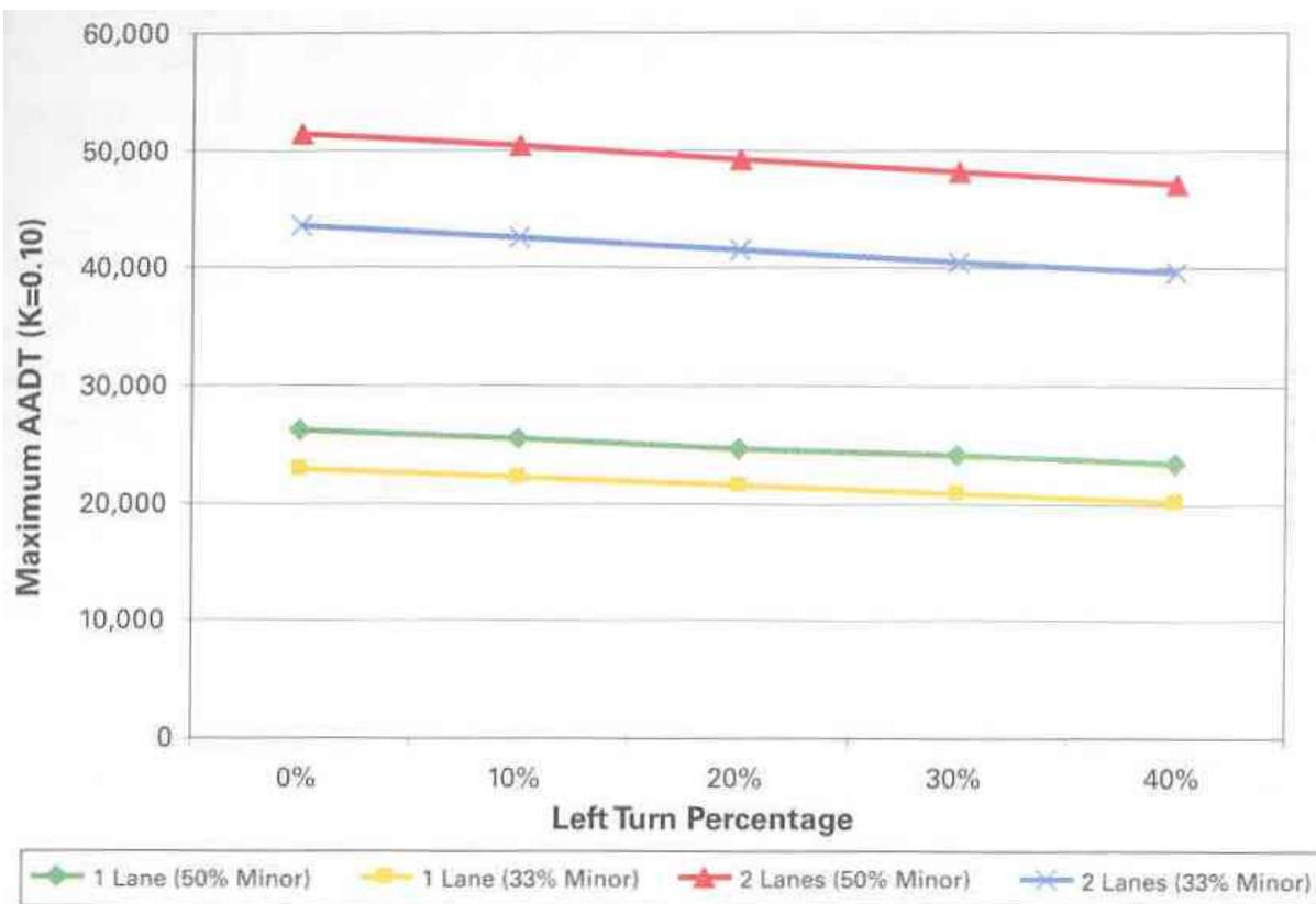
Exhibit 10: Capacity of single- and double-lane roundabouts. (source: Roundabouts: An Informational Guide, FHWA)
