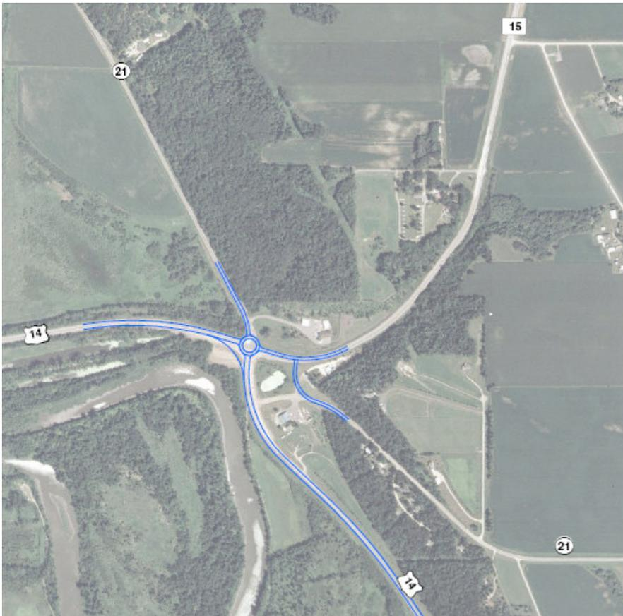
**Exhibit 12:** Four-leg roundabout with the connection to CR 21 provided along MN 15. This intersection location is not optimal due to the steep grade on MN 15.
